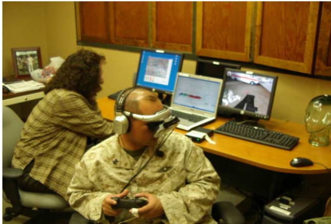
Figure 1. Three computer configuration for VR-GET with Biofeedback being calculated on the laptop computer. Simulated patient is holding a hand-held controller that he is using to “move” through the combat environment. A Head Mounted Display and Headphones facilitate the immersion in the VR-GET simulated combat environment.
