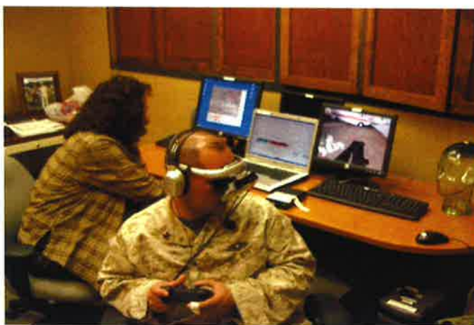
Figure 1. Three computer configuration for VR-GET with Biofeedback being calculated on the laptop computer. Simulated patient is holding a hand-held controller that he is using to “move” through the combat environment. A Head Mounted Display (HMD) and Headphones facilitate the immersion in the VR-GET simulated combat environment.
